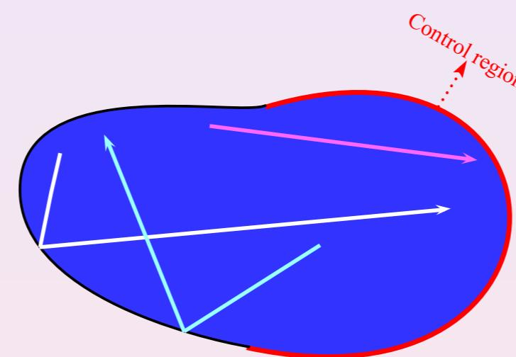
*Rays propagating inside the domain  $\Omega$  following straight lines that are reflected on the boundary according to the laws of Geometric Optics. The control region is the red subset of the boundary. The GCC is satisfied in this case. The proof requires tools from Microlocal Analysis.*
