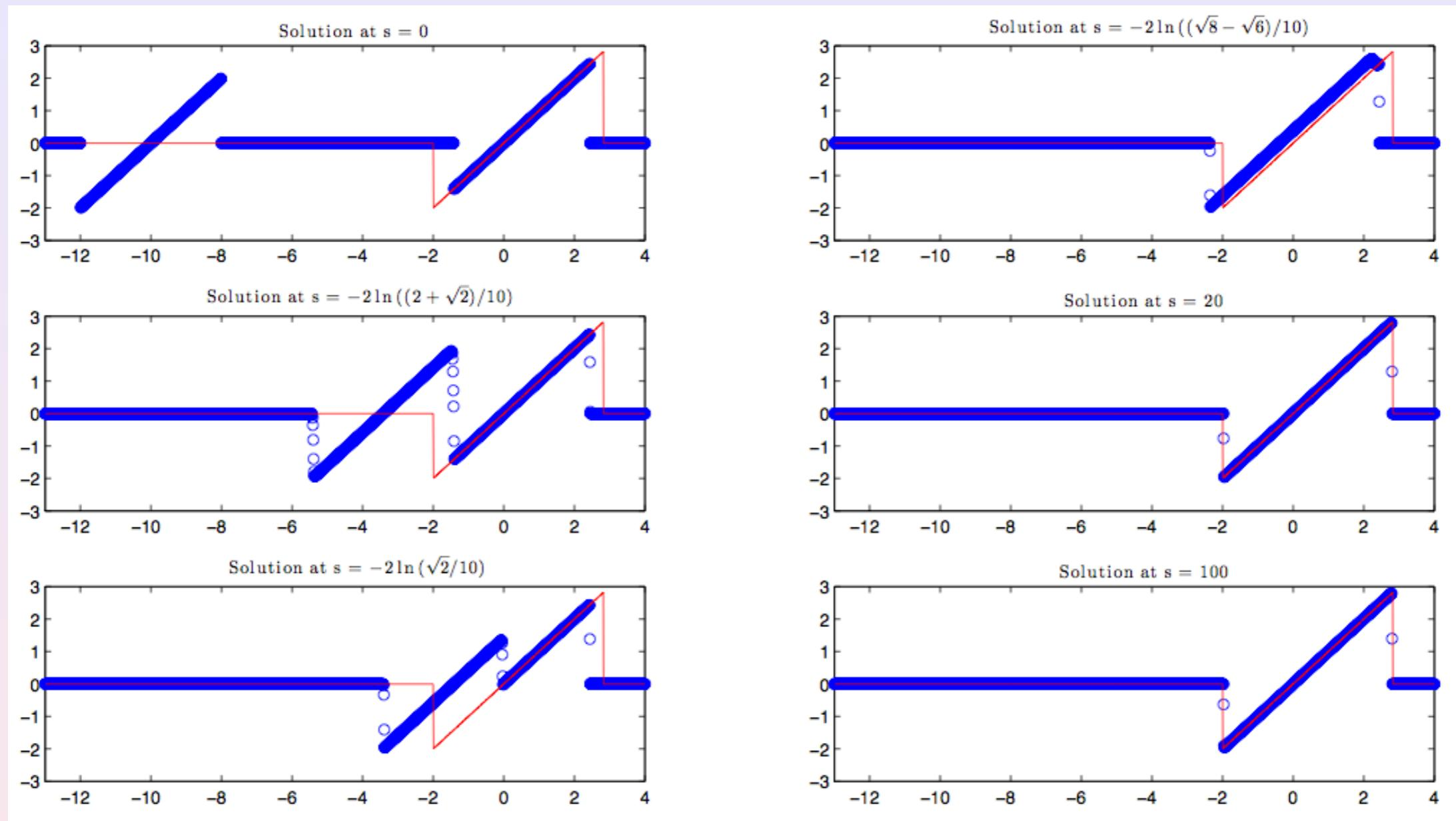
Convergence of the numerical solution using Engquist-Osher scheme (circle dots) to the asymptotic N-wave (solid line). We take  $\Delta\xi = 0.01$  and  $\Delta s = 0.0005$ .
