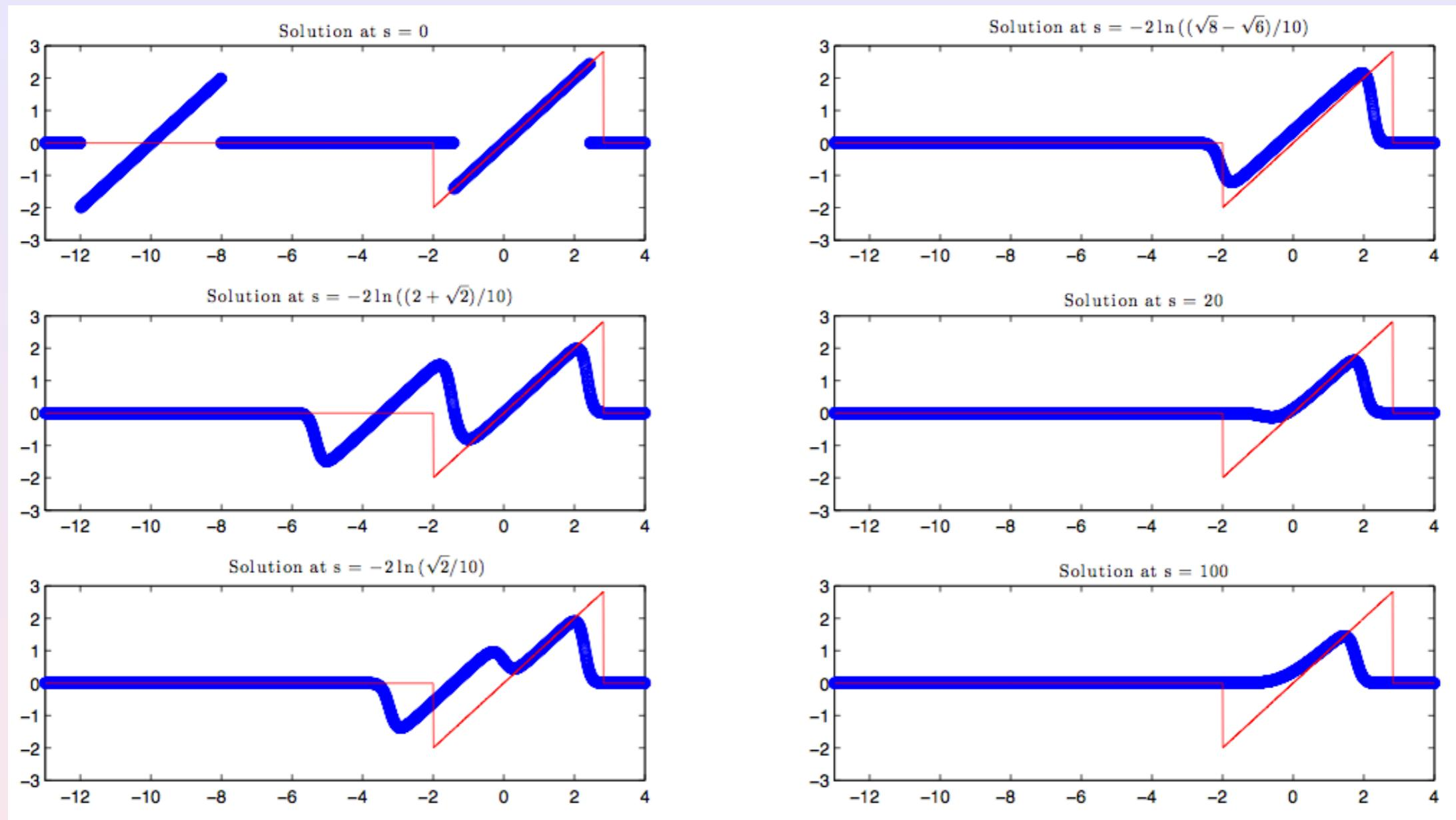
Numerical solution using the Lax-Friedrichs scheme (circle dots), taking  $\Delta\xi = 0.01$  and  $\Delta s = 0.0005$ . The N-wave (solid line) is not reached, as it converges to the diffusion wave.
